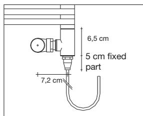
Kit for ROOM THERMOSTAT kit with Class 2 electric resistor (code ZRES#S8 or S9) supplied with an additional charge in price
